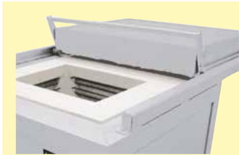
Pit-type furnace S 73/HS with rolling lid
