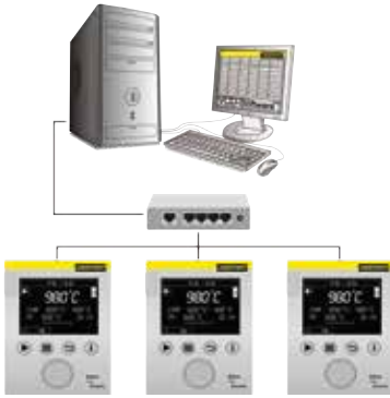
Example lay-out with 3 furnaces
