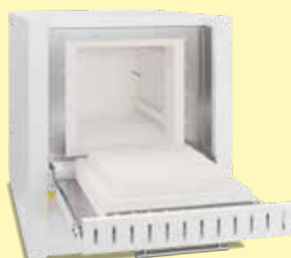
Muffle furnace LE 14/11
