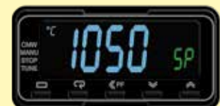
Example of an over-temperature limiter
