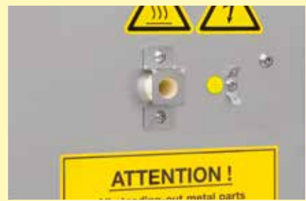
Ashing furnace LV 5/11 with port for thermocouple in the rear wall of furnace
