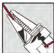
Draht abmessen und trennen Measuring and cutting of wire to length
