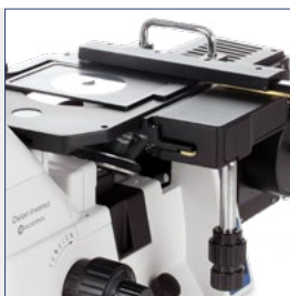
Large stage with X-Y mechanical stage
