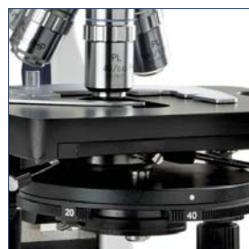
Zernike phase contrast condenser with filter holder
