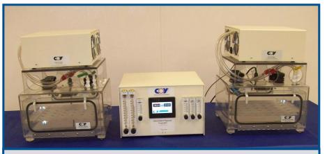
Cabinets and Gas Exchanger are put inside the incubator/oven, while the IH Controller – Model P (center) is outside.
